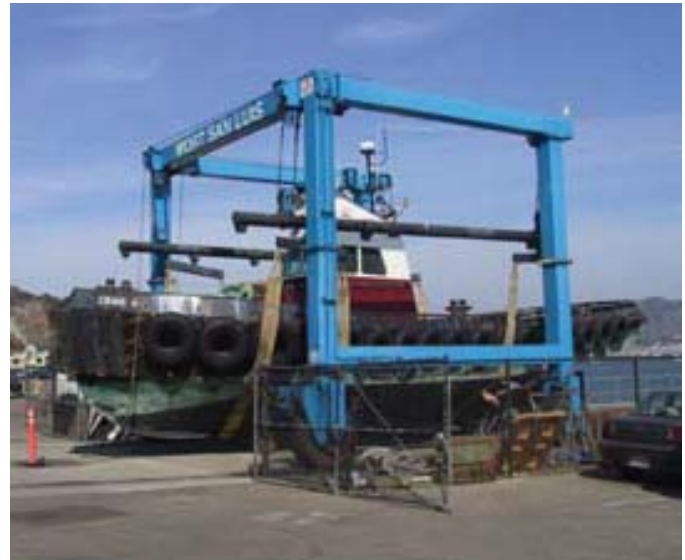
Mobile boat hoist at Harford Landing.
